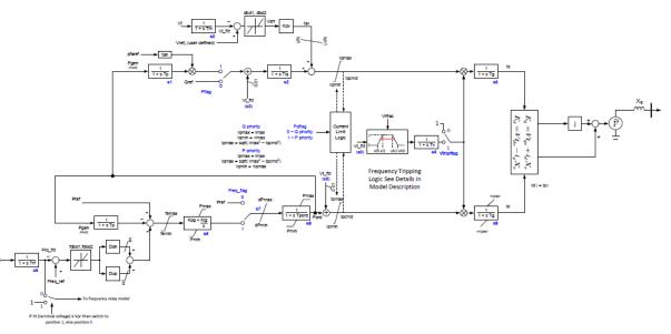
Figure 2: Proposed distributed energy resource model version A (DER\_A).
